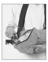
4. Open the high-pressure gas cylinder valve.
